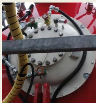
*The main visible difference between SyreN+ and the conventional SyreN system is that the slurry tanker has an in-built tank for liquid ammonia, here seen from the rear end of the slurry tanker.*
